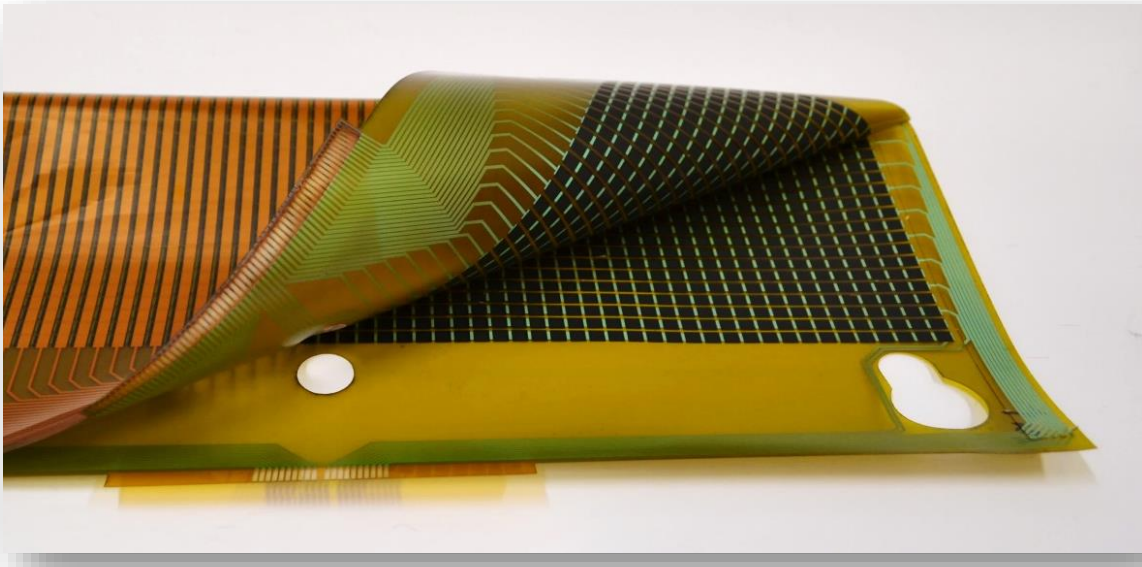
Matrix of printed piezoresistive pixels on thin polyimide substrate.
